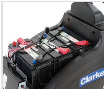
Batteries Choose between wet cell or service-free AGM batteries.
