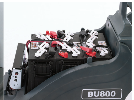
Choose between wet cell or service-free AGM batteries. Onboard charger is standard.
