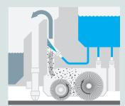
Dry Sweep Mode with dual brushes for daily sweeping and two-stage filtration for complete dust containment
