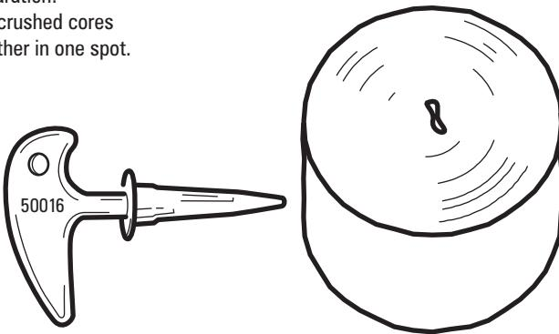
**2** Next comes reforming: Hold and compress (i.e. squeeze) each crushed roll to open the core.
