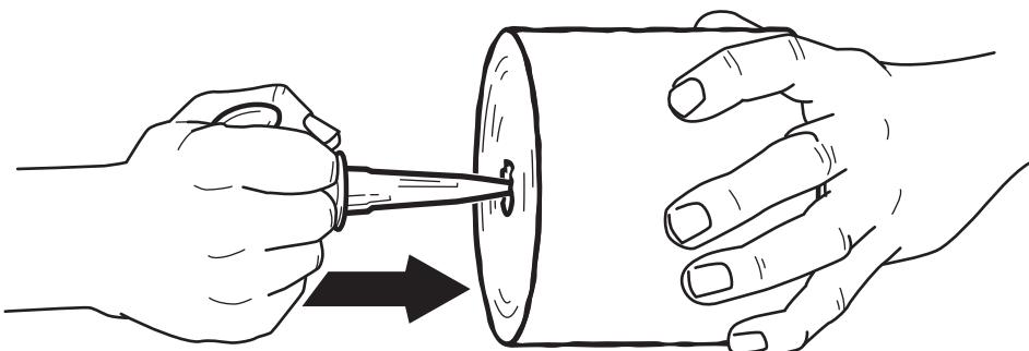
**4** Push the tool until it stops, remove the tool and repeat the action from the other end of the core.
