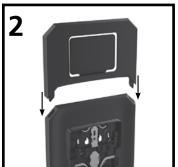
Slide two prongs at the bottom of the MESSENGER Dispenser Station into the inlet holes above TRUE FIT Wall Plate until they set in. The MESSENGER Dispenser Station accepts a standard 3"x4" clear name badge holder with a 3"x 4" name badge card that can be ordered from most office supply vendors. Print a message on a 3"x 4" name badge card and insert the message between the frame and back with message facing out.
