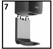
Install the SHIELD™ Floor and Wall Protector into the bottom of the dispenser by aligning plastic tabs on the Shield with slots on the dispenser and sliding up until the tabs snap into place. (Shield is included with Sanitizer Systems and can be ordered for Soap systems). 7745-WHT-18 White SHIELD Floor and Wall Protector 7745-GPH-18 Graphite SHIELD Floor and Wall Protector
