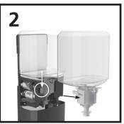
Push Release button and remove empty refill.
