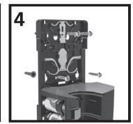
Using dispenser as a template, mark and drill four holes using 1/4" drill bit. Use the supplied #10 x 1" screws to secure the dispenser in place, being careful not to over tighten. It is recommended to use 4 screws however if only two are possible, the top two should be used.
