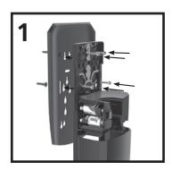
Install the TRUE FIT wall plate at the designated anchor holes.
