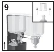
Remove refill cap and push the new refill into dispenser until it clicks in place. Close dispenser cover. The green Status light will blink after closing, indicating the dispenser is ready to use.
