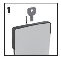
Open a locked dispenser by inserting the key into the key hole on the top of the dispenser to release the front cover.
