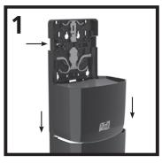
Open dispenser by pressing release buttons on side of dispenser and slide the front cover down.
