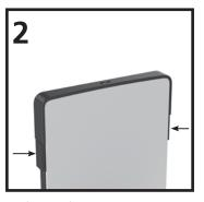
Check for a successful lock by pressing the release buttons on side of dispenser to see if the front cover releases and slides down. Once locked, the dispenser will remain in the locked state.
