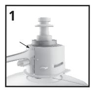
Insert a flat blade screwdriver into the slots on the refill collar and twist to separate the collar from the refill. Unscrew the pump from the bottle and discard.
