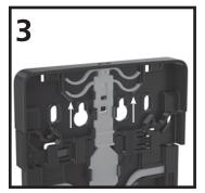
Restore to the unlocked position by pushing the locking mechanism toward the top of the dispenser.
