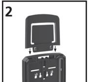
Slide two prongs at the bottom of the MESSENGER Dispenser Station into the inlet holes above TRUE FIT Wall Plate until they set in. The MESSENGER Dispenser Station accepts a standard 3"x4" clear name badge holder with a 3"x 4" name badge card that can be ordered from most office supply vendors. Print a message on a 3"x 4" name badge card and insert the message between the frame and back with message facing out.
