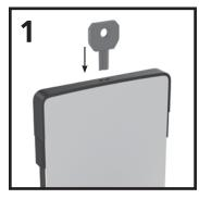
Lock the dispenser by aligning the key with the key hole on the top of the dispenser and push down until a click is heard
