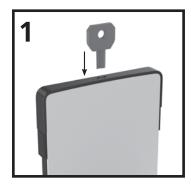
Open a locked dispenser by inserting the key into the key hole on the top of the dispenser to release the front cover.
