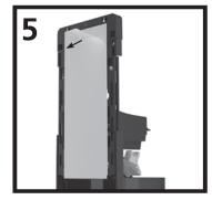
Clean installation surface with an alcohol pad. Allow surface to dry for 60 seconds then peel paper off installation tape and press firmly on back plate for 10 seconds. For maximum adhesion, wait 24 hours before loading refill or applying significant force.
