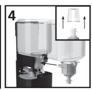
Remove refill cap and push the new refill into dispenser until it clicks in place.
