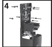
Using dispenser as a template, mark and drill four holes using 1/4" drill bit, Use the supplied #10 x 1" screws to secure the dispenser in place, being careful not to over tighten. It is recommended to use 4 screws however if only two are possible, the top two should be used.
