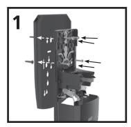
Install the TRUE FIT wall plate at the designated anchor holes.
