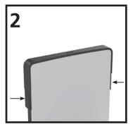
Check for a successful lock by pressing the release buttons on side of dispenser to see if the front cover releases and slides down. Once locked, the dispenser will remain in the locked state,
