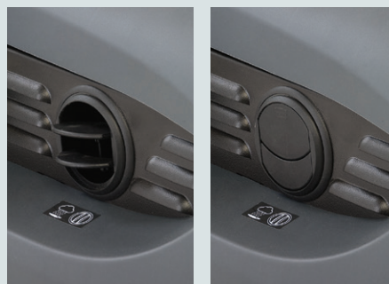
Wet sweep bypass protects the filter from water fouling when sweeping in wet conditions.
