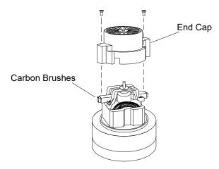
If armature commutator is grooved, extremely pitted or not concentric, the motor will need to be replaced or sent to a qualified service center.
