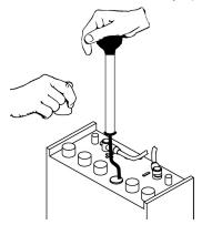
NOTE: Do not take readings immediately after adding distilled water, if the water and acid are not thoroughly mixed, the reading may not be accurate.
